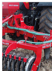
Band seeding before the packer roller
