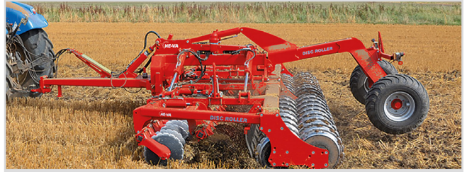
8.00 m Disc-Roller Contour with V-Profile roller and support wheels.
