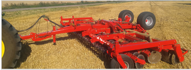
5.50 m Disc-Roller Contour with Twin V-Profile roller and material damper guard.
