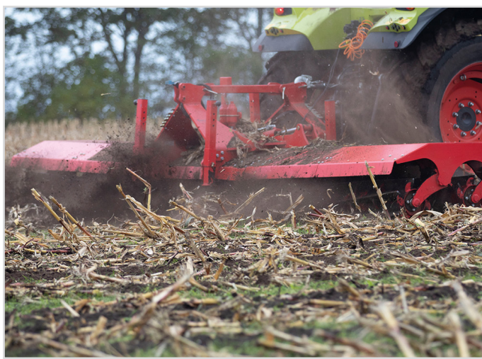
Three-point linkage on Top-Cutter Solo, enabling both front- and rear mounting
