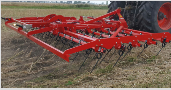
6.00 m Top-Strigle with 5 rows and 16 mm tines
