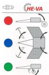
Identification marks for the machine's hydraulic system:
