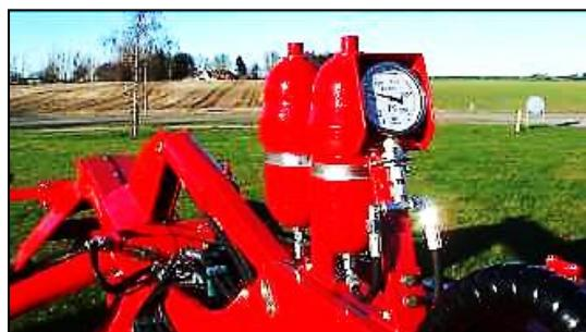
**Manometer for pressure adjustment on 2-sections machines**
