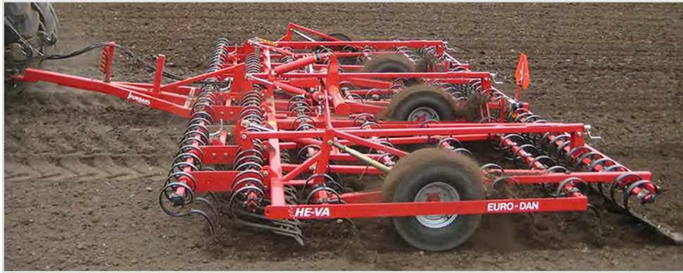
Euro-Dan Eco 8.00 m with Strong front-harrow, Spring-Board spring tine levelling bar and Spring-Board after-harrow.
