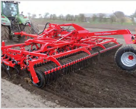
7.50 m trailed Terra-Dan MKII with V-Profile Roller.
