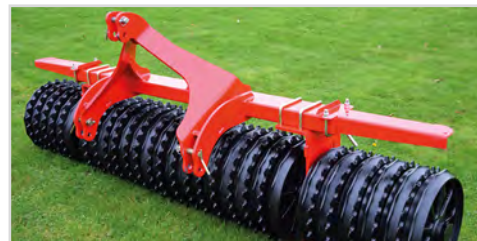
Front-Roller with fixed three-point hitch - not self-steering.
