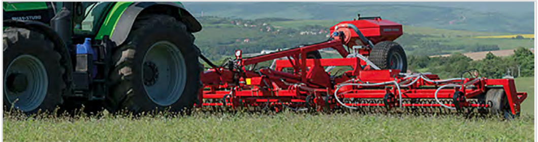
6.30 m Grass-Roller Ø710 mm with package 3 and Multi-Seeder.
