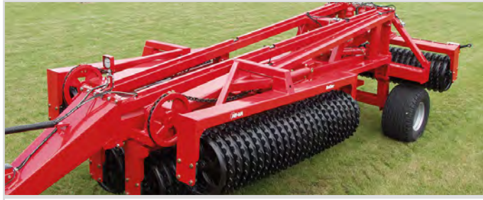
King-Roller 15.30 m. mounted with 620 mm/24" Cambridge rings.
