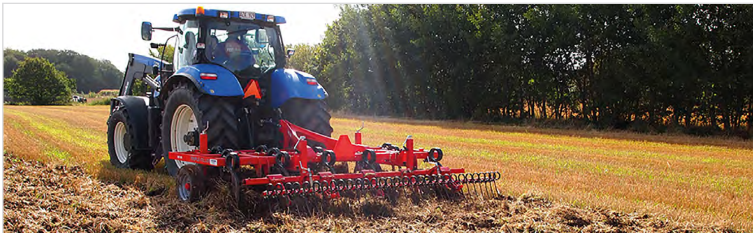
4.00 m Triple-Tiller Airy with spring tines.
