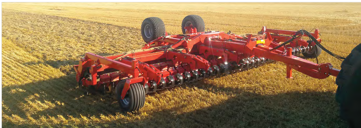
6.50 m Disc-Roller Contour with V-Profile Roller, material damper guard, pivoting support wheels and two-point pivoting crossbar.
