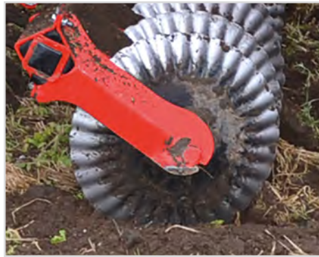
Ø570 x 5 mm profiled mixing disc.
