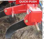
The Quick-Push shear bolt breaks if a tine hits a stone. Then the R-clip is removed and the shear bolt is easily pushed forward into new position.
