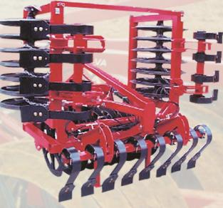
Front-Pakkers are available as 1.50 - 4.00 m rigid models or as 4.00 - 6.00 m hydraulic folding models.
