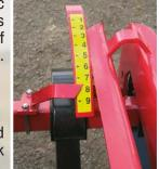
The numbered gauge that can be viewed from the tractor seat sets the angle of work or the conditions in hand.
