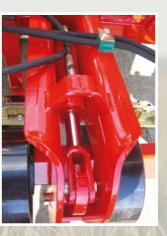
All machines that incorporate a Spring-Board have hydraulic adjustment of the working depth, so that the aggressiveness can be adjusted on the move or the Spring-Board lifted out of work completely if the conditions dictate.
