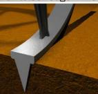
penetration with the shoulder at the base of the cutting edge.
