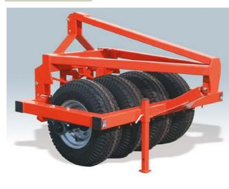
Where a precisely uniform consolidation between the tractor's tyres and either side of the tractor wheels is requested, the Press-Roller with rubber wheels will be the ideal solution. The 4.00 m model is equipped with a wheel on both sides consolidating the soil outside the area where the tractor's wheels and/or twin wheels will consolidate.
