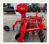
For weight distribution reasons, the optional Multi-Seeder is centrally placed on the roller.
