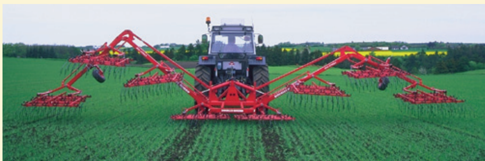
12 m model: demonstration of the folding system in field.
