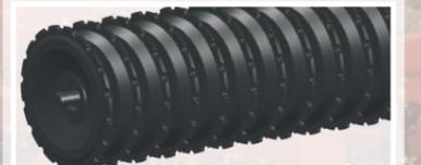
Ø600 mm packer roller cuts through the surface, leaving an ideal consolidation and - more importantly - a weatherproof surface. The Ø600 mm V-profile is a serrated ring of pressed steel with a shoulder profile that easily breaks clods on heavy soils and consolidates lighter soils efficiently. Effective scrapers mounted between the rings make an even consolidation possible in all soil conditions.
