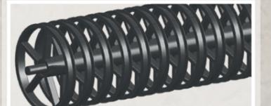
The U-profile roller is designed so that the roller fills with soil when at work. This ensures a good soil-to-soil consolidation and gives the soil surface a natural structure.
