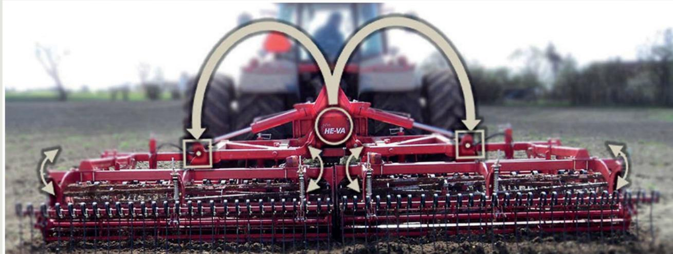
The HE-VA Terra-Dan MKII is unique thanks to the 2 completely independent centre-pivoting wing sections. The harrow is extremely flexible on hilly surfaces, not to mention consolidates the soil evenly across the working width by transferring the weight of the frame, wheel frame and drawbar (o) onto the centre of each section (see photo).
