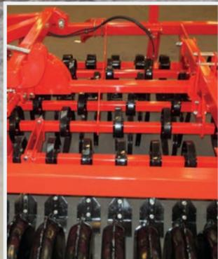
45x12 mm tines with 8.5 cm row spacing for a fine and uniform seedbed preparation.
