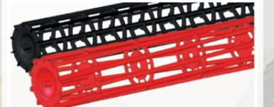
Ø550/Ø410 mm double roller consisting of a Ø550 mm square tube roller followed by a Ø410 mm flat bar roller. The square tube roller consolidates the surface, and the flat bar roller then acts as a powerful rotor crumbler, making the double roller ideal for heavier soil types, as the surface will have a very fine structure.
