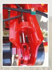
All machines that incorporate a Spring-Board have hydraulic adjustment of the working depth, so that the aggressiveness can be adjusted on the move or the Spring-Board lifted out of work completely if the conditions dictate.
