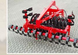
4,00 m Spring-Board for 1.65 m Front-Pakker has as standard mechanical change-over into a transport width of 2.85 m.
