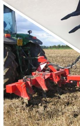
The quick couplings allow the HE-VA Combi-Tiller MKI to be built together with another three-point mounted implement, for example the HE-VA Disc-Roller.
