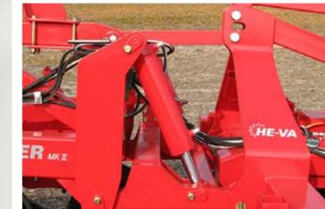
Hydr. three-point linkage is standard equipment on the Combi-Tiller MKII. It allows the Combi-Tiller MKII to be mounted with a trailed implement directly in the three-point linkage Cat. 2/3. The linkage will then act as a hydr. depth adjustment of the Combi-Tiller MKII tines.
