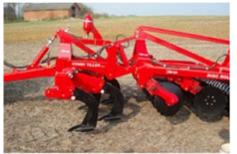
When combined with a HE-VA Disc-Roller, the tine working depth can be adjusted from 50 mm above the soil surface to a max. depth of 400 mm.
