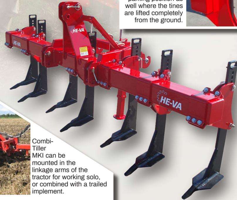
Combi-Tiller MKI can be mounted in the linkage arms of the tractor for working solo, or combined with a trailed implement.
