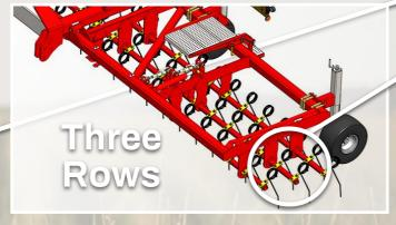
The HE-VA Grass-Combi is available with either two or three rows of tines. The two-row model is recommended for smaller tractors due to the lower lifting requirement. The 3-row variant, on the other hand, offers increased work intensity due to the number of tines.
