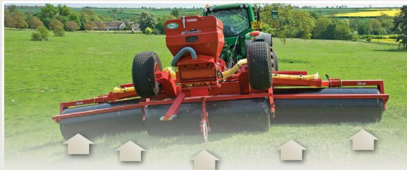
The centrally pivoted side sections are, with the help of support arms, ensured free movement in relation to the mid section. At the same time, the mid section can follow the field's contours independently of the tractor, as the drawbar is equipped with a rotatable prod eye. All of this combined makes the roller's three sections completely flexible in relation to the field's surface.
