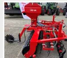
For weight distribution reasons, the optional Multi-Seeder is centrally placed on the roller.
