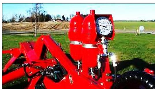
Manometer for pressure adjustment on 2-sections machines
