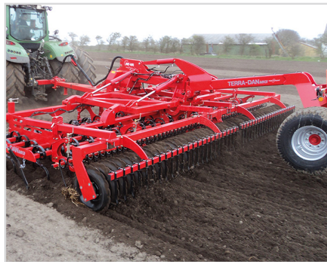
7.50 m trailed Terra-Dan MKII with V-Profile Roller.
