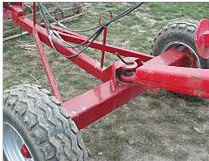
Dolly: wheel set making an attachment of rollers possible behind a harrow - 11.5/80 x 15.3 wheel.
