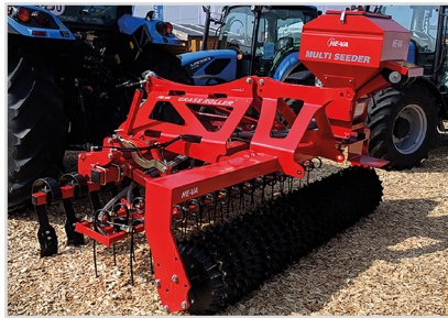
2.90 m three-point mounted Grass-Roller with Star rings and equipment package 4.
