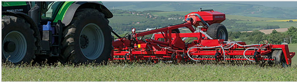
6.30 m Grass-Roller Ø710 mm with package 3 and Multi-Seeder.
