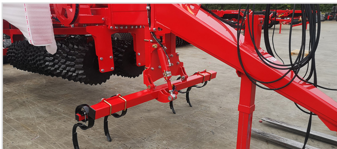
Wheel track eradicator, hydraulically adjustable
