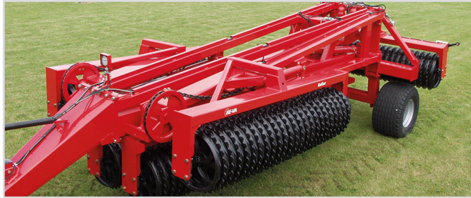
King-Roller 15.30 m. mounted with 620 mm/24" Cambridge rings.
