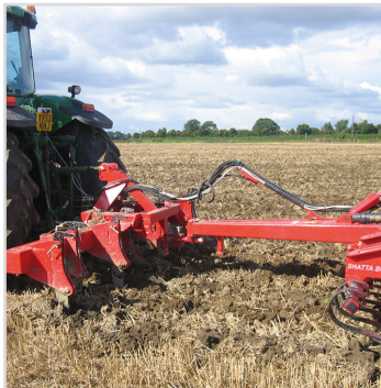
Combi-Tiller MKI with three-point linkage for combination with several lift mounted/trailed implements. E.g. bed formers for potatoes or trailed drill units.
