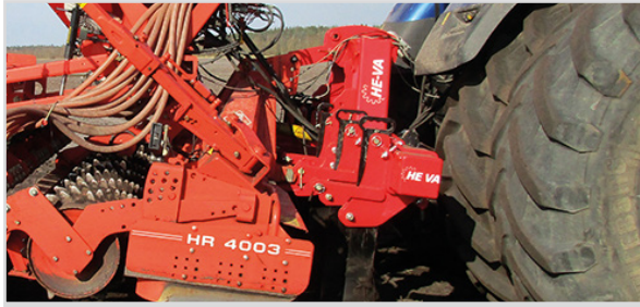
4.00 m Combi-Tiller PTO with 5 tines.
