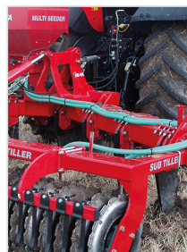
Band seeding before the packer roller
