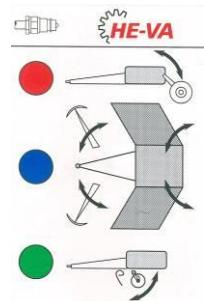
Indication label for the machine's hydraulic systems:
