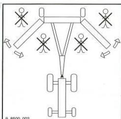
Take care that no persons are within the machine's hazardous area during the unfolding and folding procedure.
