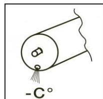
Empty the rollers of water, before the temperature is below 0 C°. If this is not observed, our guarantee obligations will no longer apply.
