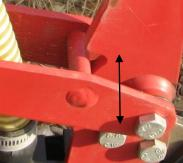
2. It is necessary to set the working height of the mounting bar each parallelogram is fitted to and therefore position of the above pin between the stops. On Trailed Hydraulic Folding machines this is set by adjusting the pairs of Top links shown in the pictures below.
