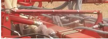
3. Seeding Depth – The Seeding Depth is determined by the relative position of the Press wheel and the Double Disc Coulter. The Press wheel is effectively the Depth control wheel for each Coulter. The Depth is adjusted using the winder which attaches the front mounting bar to the coulter bar. Shorten this adjuster and the Accu-Disc will work Deeper, Lengthen it and the Accu-Disc will work
