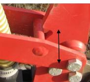
2. It is necessary to set the working height of the mounting bar each parallelogram is fitted to and therefore position of the above pin between the stops. On Hydraulic Folding machines this is set by adjusting the Hydraulic Rams show in the pictures below.
