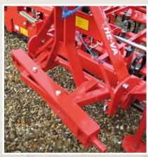
The flex drawbar on the Kulti-Dan enables halftrailing while maintaining the advantages of the lift-mounted harrow
