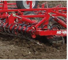
The Spring-Board is an important element on the harrow. When mounting a Spring-Board at the front of the Euro-Dan Eco. the field is perfectly levelled and major clods are crushed before the soil is culivated. The Spring-Board tine is a strong 10x45 mm spring tine, standard mounted with an 8x100 mm point.
