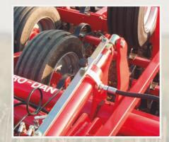
By means of a switch in the cabin. the driver can stop the electric depth stop. This way, the driver can override the stop and perform a deeper preparation - e.g. on the headlands.
