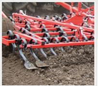
The Spring-Board after-harrow is connected to the front levelling bar, making the aggressiveness hydraulically adjustable. The ratio between the front and rear bar is adjustable via spindles.
