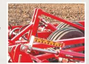
Via the scale on the right side, the driver can see exactly how aggressively the Spring-Board levelling bar is working.
