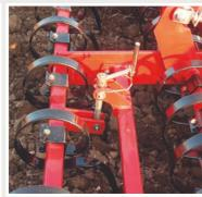
The aggressiveness (tine row angle) on the strong front-harrow is adjusted via spindles.
