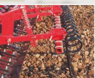
Both the pressure and the working angle is easily adjusted on the after-harrow, to achieve the desired work intensity.
