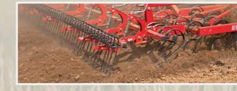
The solid longfinger afterharrow mounted with strong 12 mm back bended tines never leaves anything in bulks and it erases the harrow tine tracks effectively.
