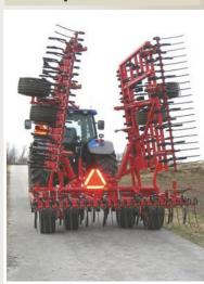
During transport the side sections are folded over into vertical position to obtain a safe and stable transport. A strong mechanical lock ensures safe movement of all units, and automatic unlocking occurs by means of the hydraulics. The strong hinge bracket for the side sections ensures high strength as well, when the harrow is in working position.
