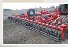
A flat bar roller Ø400 mm mounted with the longfinger harrow in front leaves a pulverized and light consolidated surface. With its construction of 8 x 40 mm flat steel, this type of roller ensures a perfect soil structure.
