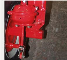
Wheel set making an attachment of rollers possible behind a harrow. Wheels: 11.5/80 x 15.3
