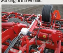
By means of a switch in the cabin, the driver can stop the electric depth stop. This way the driver can oversteer the depth stop and perform a deeper pre-
