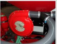
The consumption of the hydr. motor is from 10-20 l/min. The hydr. motor is equipped with a valve securing the motor against overload due to excessive oil supply
