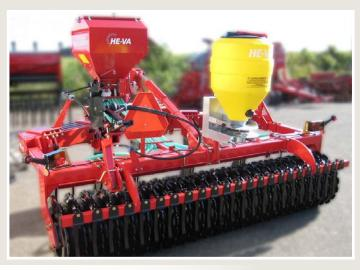
MAX-THROW always spreads with the maximum number of revolutions and contains a 90 l. tank with an electrically operated open-close function and the seed quantity is set via a hopper flap.
